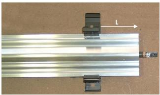
Insert the Heating Core with an aluminium profile containing armoured resistor on the brackets (art.OE), making them slide on the specific place as indicated on the drawing.
