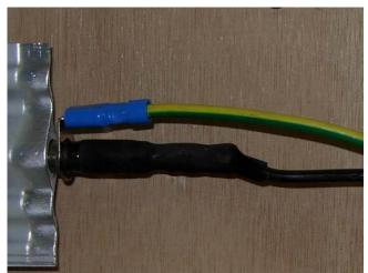
Insert the thermotight pipe on high temperature wire (silicon type). Proceed with parallel electrical connections, use faston in equipment.
