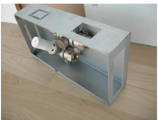
Unpack the equipment and check that the arrow on the valve point in the same water direction. If it is opposite to the expected one, unscrew the valve and holder from the collars and turn them.
