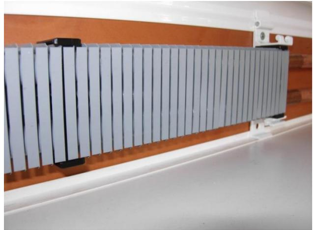
Before placing the heating core on the brackets and make the final connections, be sure that there are no blades ( thin plates) presenting curls or folds outward. If present, both on the front and back, straighten the blades (thin plate) by pressing lightly with your finger, or, if they are difficult to bend push slightly to the inside of the heater core.
