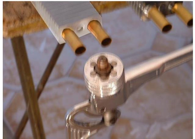
Clean the end of the copper heating core thoroughly with steel wool before soldering
